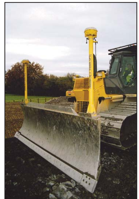
"The Site Positioning System was used to validate output, and to see how close the operator is to final grade"
